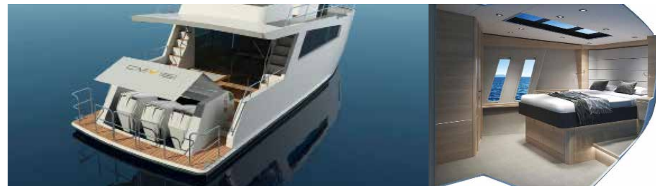
BELOW Triple Oxe 300hp diesel outboards give up to 27 knots and a range of 3,000nm
